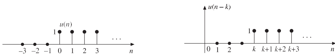
Figure 1.3 Discrete-time (a) Unit step function (b) Shifted unit step function
