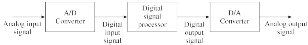
Figure 1.1 Block diagram of a digital signal processing system.
